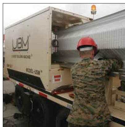
A Marine with Marine Wing Support Squadron 172's combat engineer platoon guides a piece of steel through the Ultimate Building Machine — a mobile device used to rapidly build various steel structures — during training on the device Feb 6.
